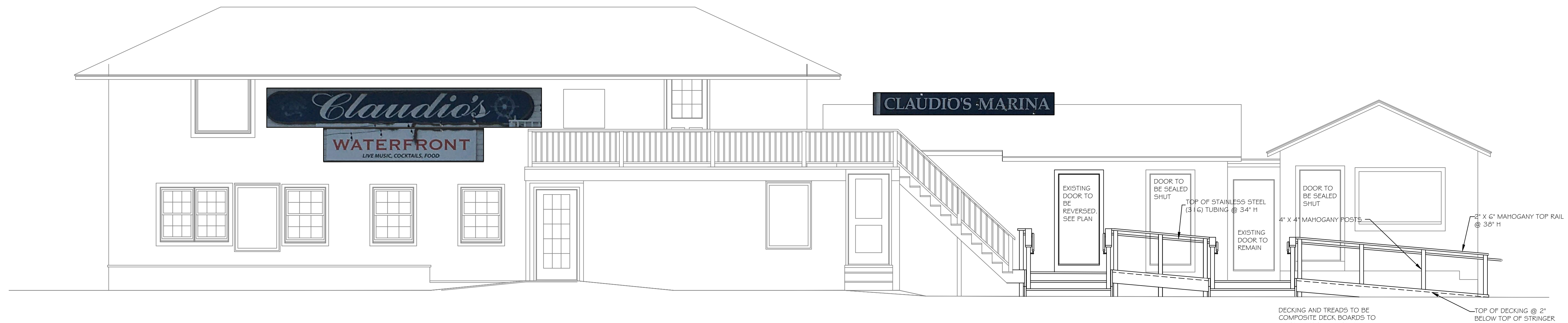
EXISTING EAST ELEVATION WITH PROPOSED ACCESSIBLE RAMP
